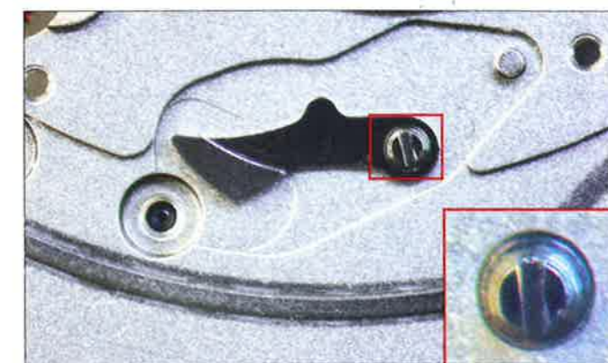
Figure 9. The date jumper pivot is eccentric, for fine adjustment to the date display.
